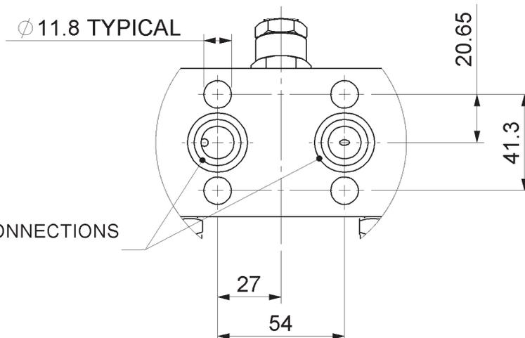
MANIFOLD INSTRUMENT CONNECTIONS
