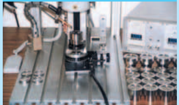
Laser welding of diaphragms.
